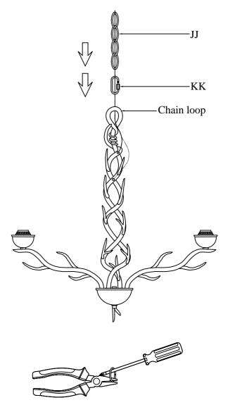
To open a chain link: Use a pair of pliers and a screwdriver as shown above to open a chain link. Wrap the jaws of the pliers with cloth to protect the finish of the chain.
